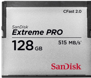
Figure 3 Showing one example of the newly standardized CFast (2.0) memory cards
