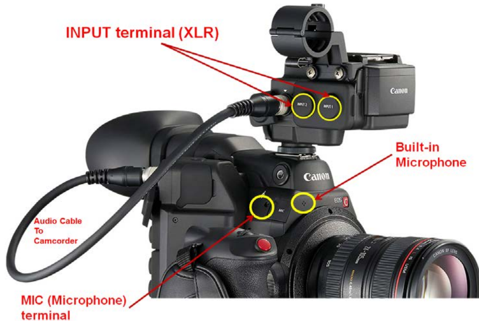
Figure 6 Showing the four separate audio inputs to the C300 Mark II
