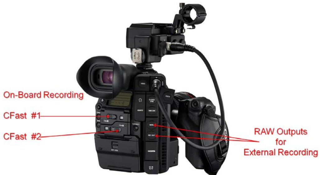
Figure 5 Showing the two CFast cards for on board recording and the two RAW outputs for external recording
