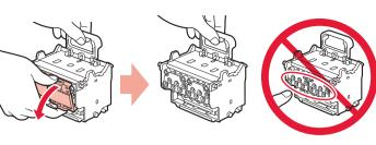
EN Close the print head lock lever (B) and joint lever (A).
