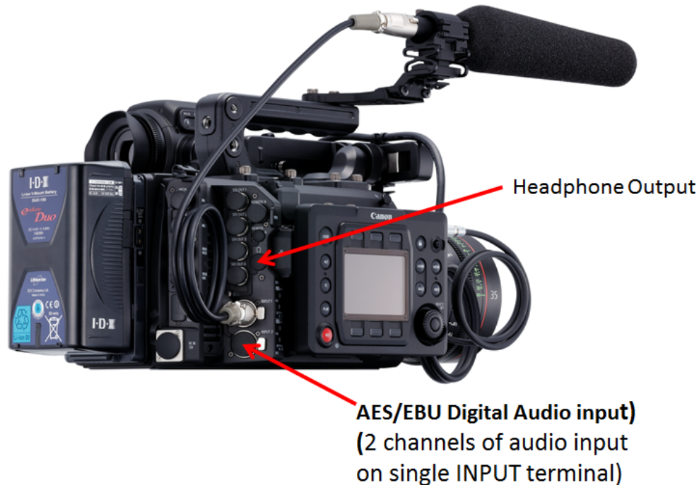
Figure 8 Showing the audio inputs to the C700
