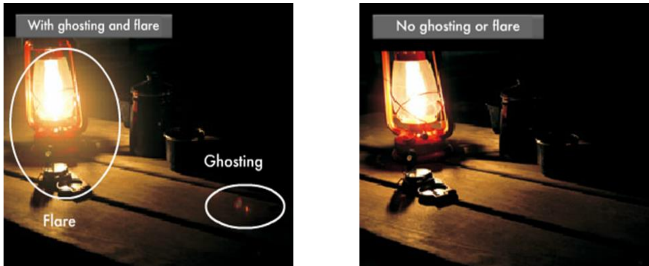
Figure 4 Examples of glare and ghosts within a lens caused by unwanted reflections and their effective elimination with high quality optical coatings
