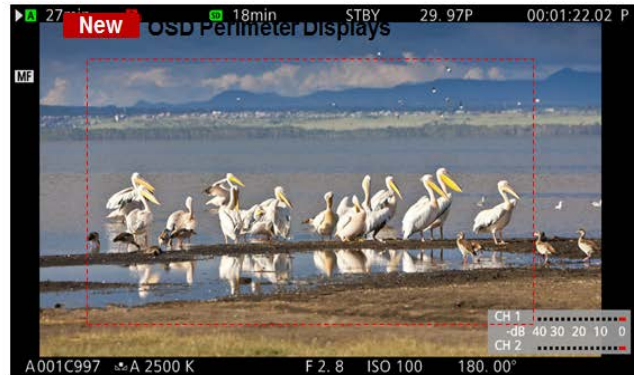
Figure 18 Comparing the salient EVF image specifications of the C300 Mark II with that of the C300 on the left and showing an example of the noise-less OSD perimeter display on the right
