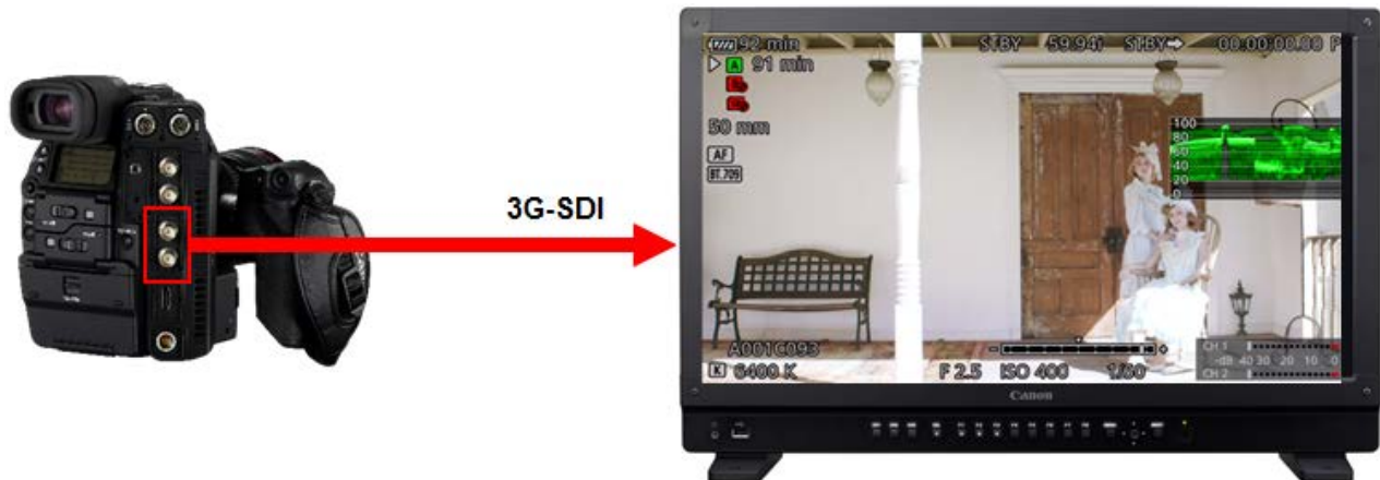
Figure 19 The Mon output 3G SDI interface and HDMI interface carries certain camera assist information and the WFM to the external display.
