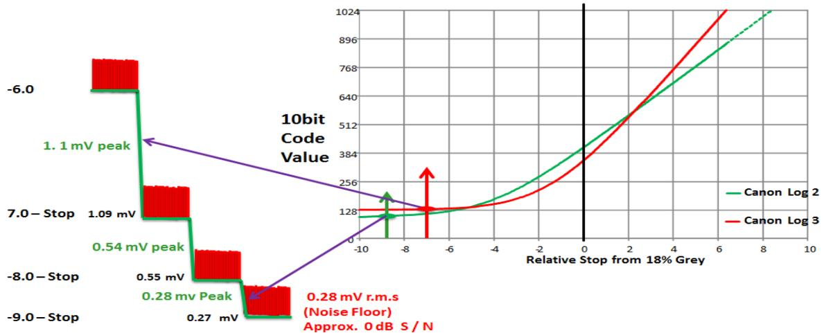
**Figure 3** Shows the lower T-Stops signal level capability of the EOS C300 Mark II image sensor and where they align with the Canon Log curves
