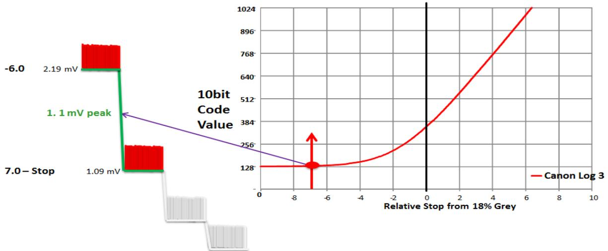
**Figure 8** *Showing the curtailment of the lower end of Canon Log 3 curve and how it eliminates signals below the -7.0-Stop level*
