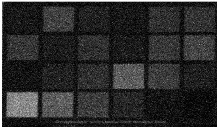
**Figure 6** *A test chart with close to unity signal to noise ratio (0 dB S/N) at the lowest black level*
