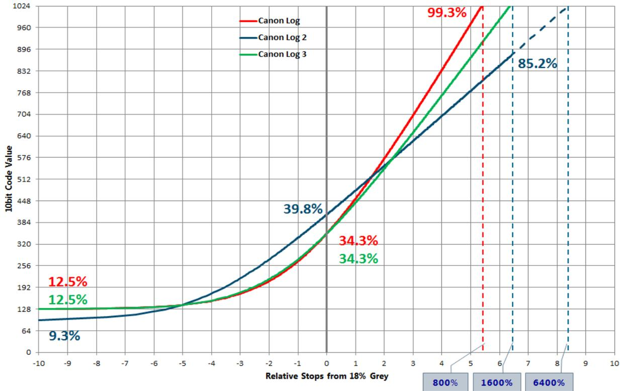
**Figure 2** Showing the same three Canon Log curves in semi log form
