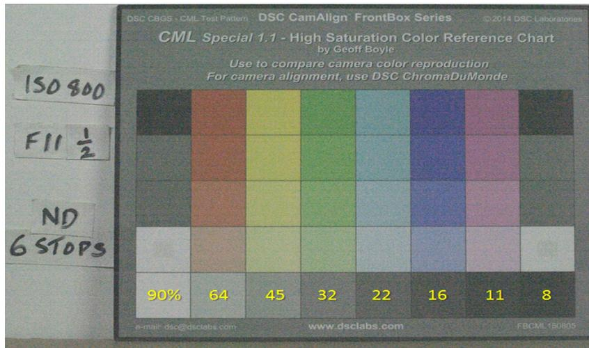
**Figure 5** *A 6-stop ND filter switched into a nominally exposed chart places the black chip at 9.5 stops below 100 IRE reference white level*
