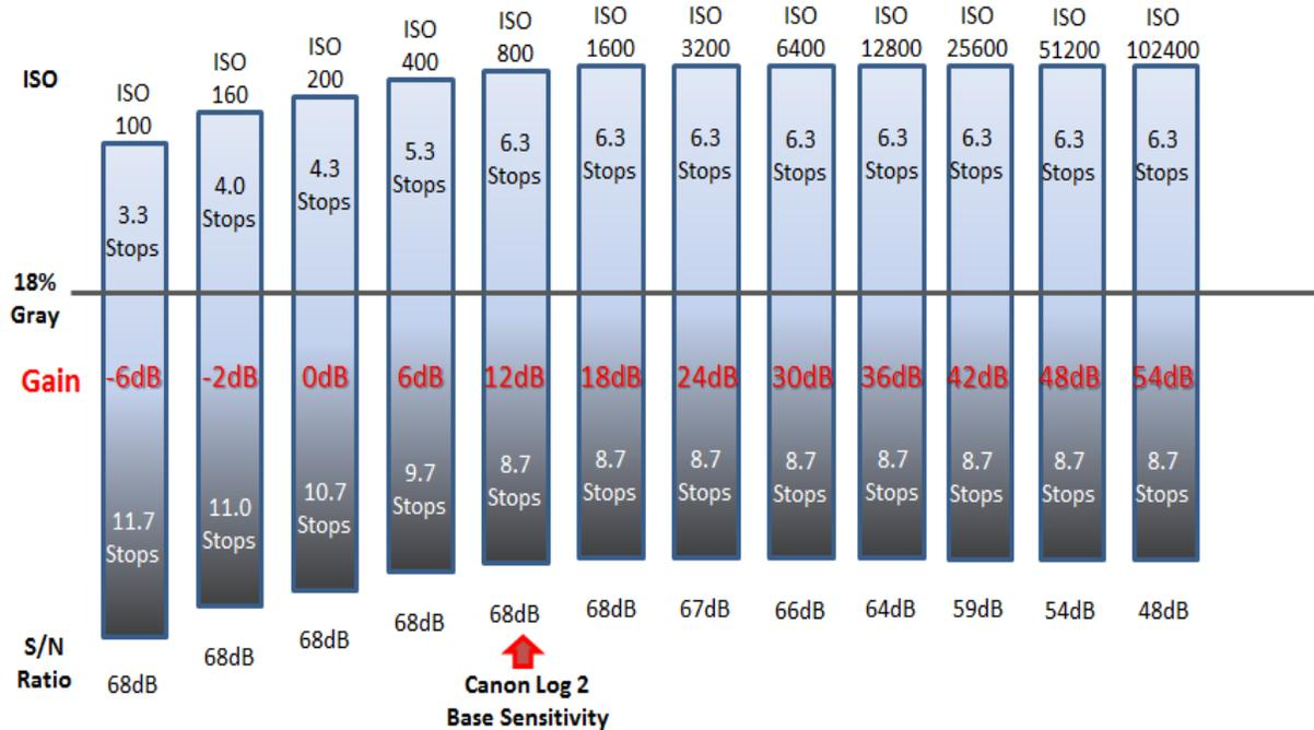
**Figure 9** The Sensitometric characteristic with increasing ISO settings for the C700 camera
