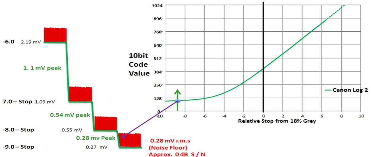
**Figure 4** The Canon Log 2 extends almost 9-Stops below reference 18% gray and accordingly it reproduces the image sensor level where the S/N becomes approximately unity
