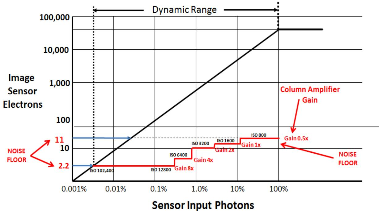
**Figure 10** Increasing the amplification of the column amplifier progressively lowers the overall noise floor of the image sensor
