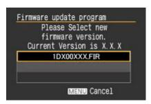
2. If you press the <SET> button, a confirmation screen will appear, so check the firmware update shown, rotate the Quick Control Dial to select [OK], and press the <SET> button again to start the firmware update.
