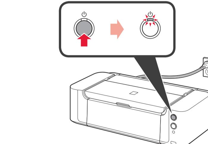
4 Press the ON button, then check that the POWER lamp lights white.
