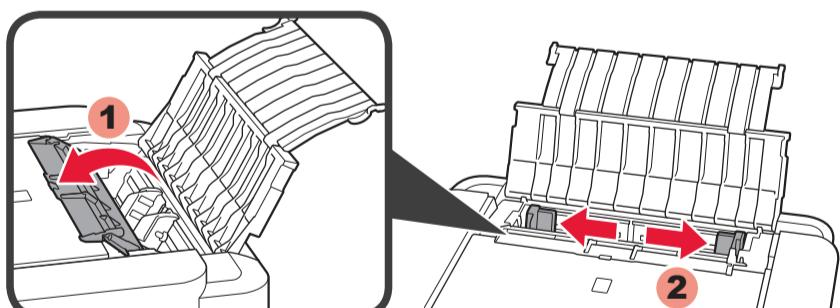
2 Open the Feed Slot Cover, then move the Paper Guide to both edges.
