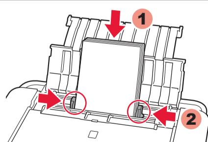
3 Load paper with the printing side facing up, then adjust the Paper Guide to fit the paper width.
