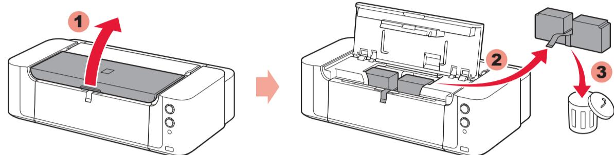
1 Open the Top Cover, then remove the orange tape and protective material.
