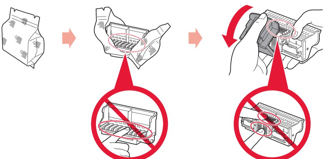
4 Take out the Print Head from the silver package, then remove the orange protective cap.
