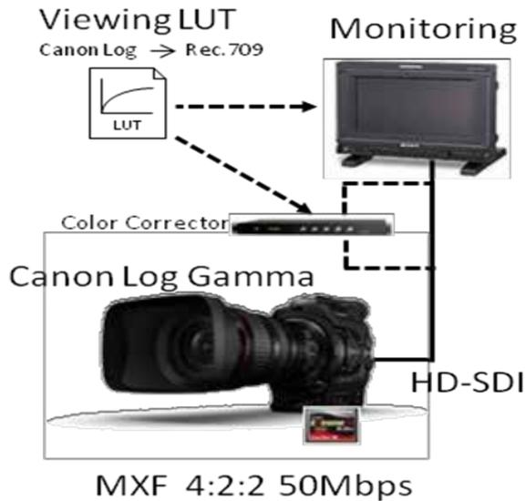
When viewing Canon-Log coded images – that are intended for theatrical release *via digital cinema projection* – on a studio reference monitor, the display LUT that is applied should emulate the contrast range and colorimetry of that digital theatrical display within the boundaries of the reference monitor.
