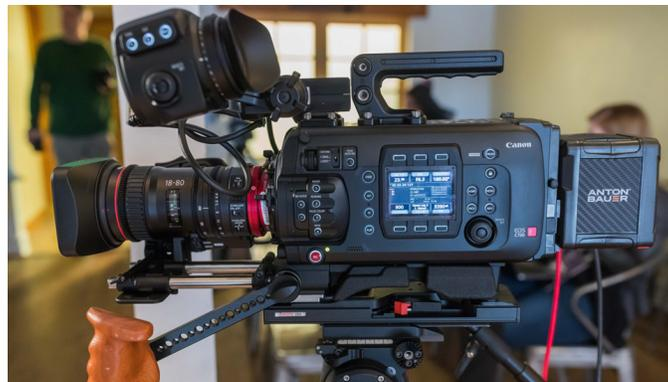
**Figure 27** *Showing a mobile EOS C700 configuration featuring the Compact Cine Servo CN-E18 – 80 mm lens*
