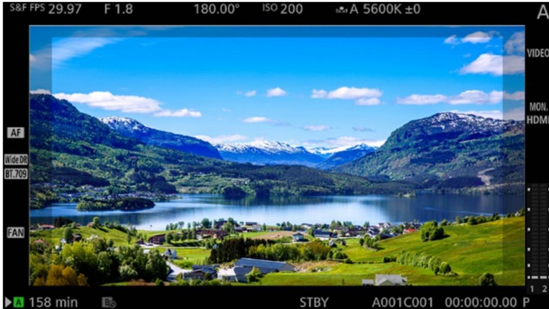
**Figure 5** With DCI viewing angle in record mode, the surround is displayed in letterbox on the 16:9 EVF panel.
