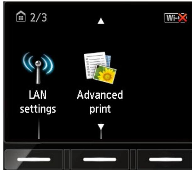
1. From the **Home** screen, press the up or down arrows until **LAN settings** appears. Then press the function key underneath it.
