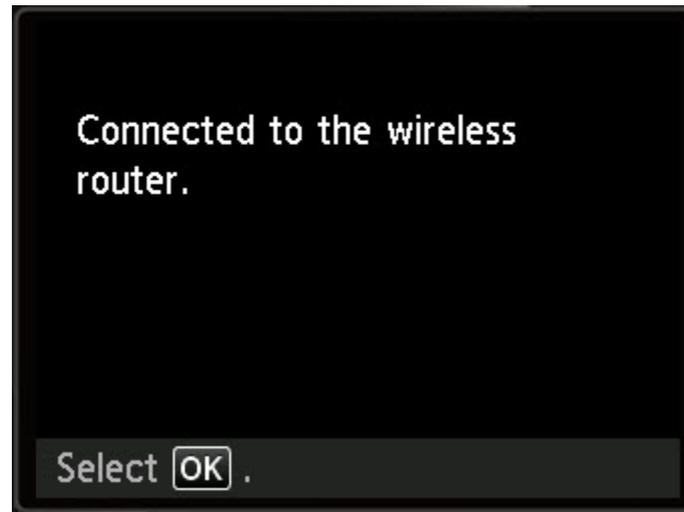
6. The printer will attempt to connect to the wireless LAN. Upon a successful connection, this screen will appear. Press **OK** and proceed with installing the software.
