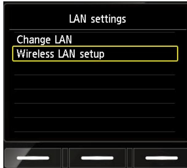
2. Use the down arrow to select **Wireless LAN setup** and press **OK**.
