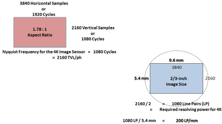
**Figure 7** On the left is the sampling structure of a 4K UHD image sensor and the Nyquist frequency associated with that sampling; the image on the right represents the spatial detail of a 4K 2/3-inch lens that can fulfill the resolution capability of that 4K image sensor
