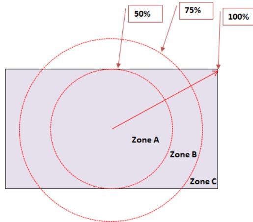
**Figure 9** The three zones used by Canon to specify levels of MTF across the UHDTV lens image plane
