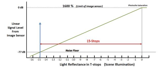
Figure 7 Showing the 15-Stop linear light transfer characteristic of the CMOS image sensor in the EOS C700 and EOS C300 Mark II cameras
