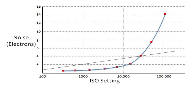
Figure 11 The behavior of EOS C300 Mark II image sensor noise over the range of ISO settings
