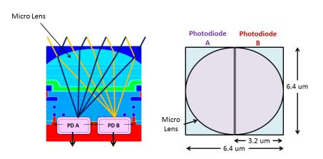
Figure 5 Showing the dual photodiode and microlens structure within a single photosite in the 4K CMOS image sensor used in the Cinema EOS cameras
