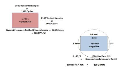
**Figure 7** On the left is the sampling structure of a 4K UHD image sensor and the Nyquist frequency associated with that sampling; the image on the right represents the spatial detail of a 4K 2/3-inch lens that can fulfill the resolution capability of that 4K image sensor
