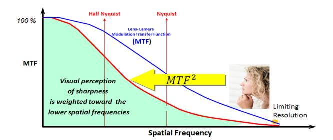
**Figure 21** Subjective image sharpness is proportional to the area under the Lens-Camera MTF<sup>2</sup> curve
