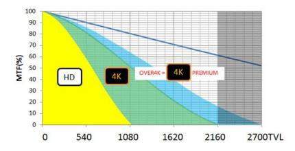
Figure 12 Showing that the 4K PREMIUM Lens has a higher MTF than the 4K lens – indicated in blue
