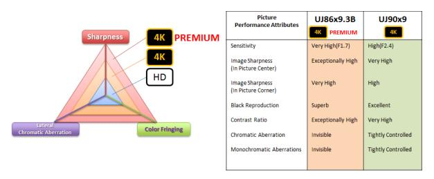
Figure 11 A simplistic overview of the critical optical design parameters that separate the overall optical performance of HD, 4K, and 4K PREMIUM
