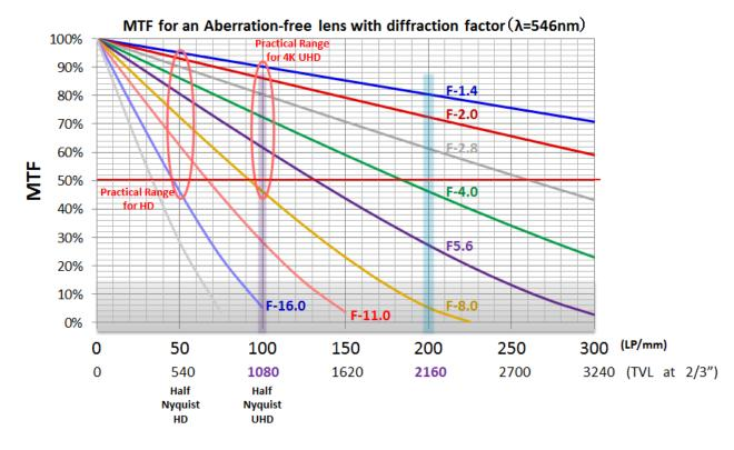
**Figure 23** Showing the effective range of lens aperture settings for the 2/3-inch lens-camera systems for HDTV and UHDTV
