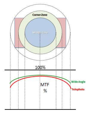
Figure 13 Showing the hypothetical MTF characteristics of a 4K lens as a function of both the two spatial zones and the total focal range
