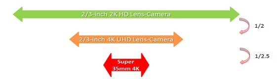
Figure 19 The 2/3-inch 4K UHD Lens-Camera imaging system will exhibit a depth of field behavior closer to that of the Super 35mm 4K UHD camera than it is to the 2K HDTV system
