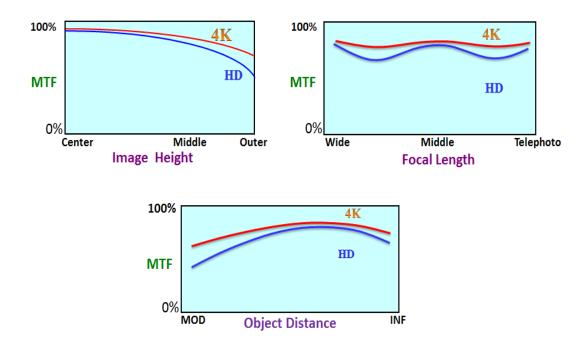
Figure 6 Simplistic illustrations of the recommendations of the 4K UHD camera manufacturers with respect to improvements to resolution in the new 4K UHD 2/3-inch lenses
